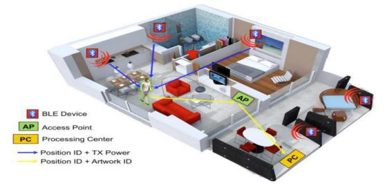
Fig 2. The components of the localization mechanism.
