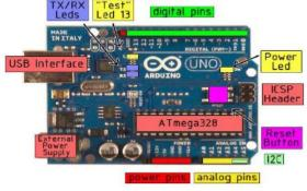
Figure 2. Arduino Uno Atmega328 microcontroller board
