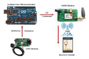
Figure 1. Block diagram of tracking and accident detection system based on GSM and GPS technology
