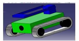
Fig 2: Mechanical design of the UGSV
