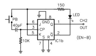
Fig 4.ID Enable Circuit B
