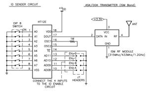
Fig 2.ID Sender Circuit
