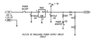
Fig 6.Power Supply to all sections of vehicle user ID circuits
