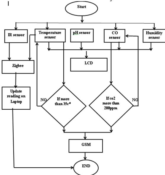
Figure 2: Flow chart of the process
